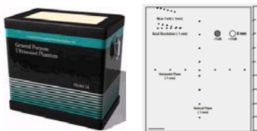
Model 054GS General Purpose Ultrasound Phantom
